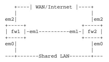
The firewalls are connected back-to-back using a crossover cable on em1. Both are connected to the LAN on em0 and to a WAN/Internet connection on em2. IP addresses are as follows:
