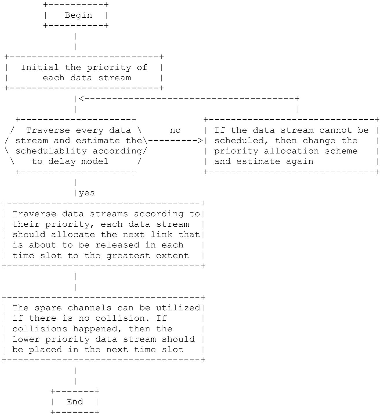
Figure 5. Scheduling of times-slotted industrial backhaul network
