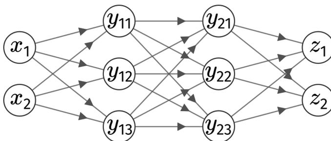
Figure 1: Graphical representation of an example dense neural network with two hidden layers  $y_1$  and  $y_2$ . Both the input layer  $x$  and the output layer  $z$  have two nodes. The input nodes can be any existing scalar CVs.
